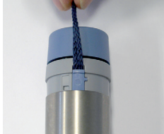
Figure (24) Assembly of the carrying strap
